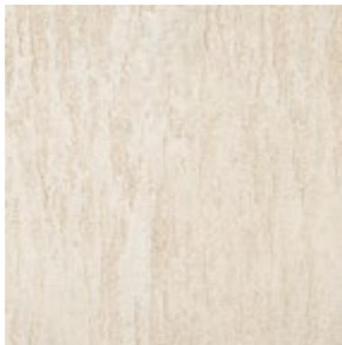
Lime-based trowel coating with marble powder for interiors and exteriors.
